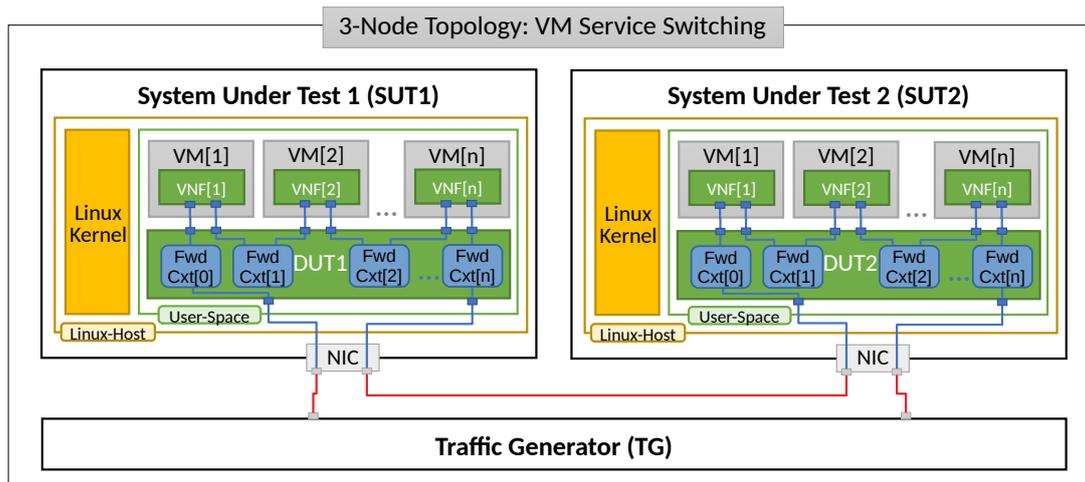
In “Chained” VM topologies, packets are switched by VPP DUT multiple times: twice for a single VM, three times for two VMs,  $N+1$  times for  $N$  VMs. Hence the external throughput rates measured by TG and listed in this report must be multiplied by  $N+1$  to represent the actual VPP DUT aggregate packet forwarding rate.
