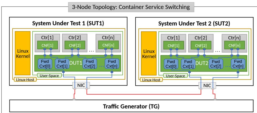
In "Chained" Container topologies, packets are switched by VPP DUT multiple times: twice for a single Container, three times for two Containers, N+1 times for N Containers. Hence the external throughput rates measured by TG and listed in this report must be multiplied by N+1 to represent the actual VPP DUT aggregate packet forwarding rate.
