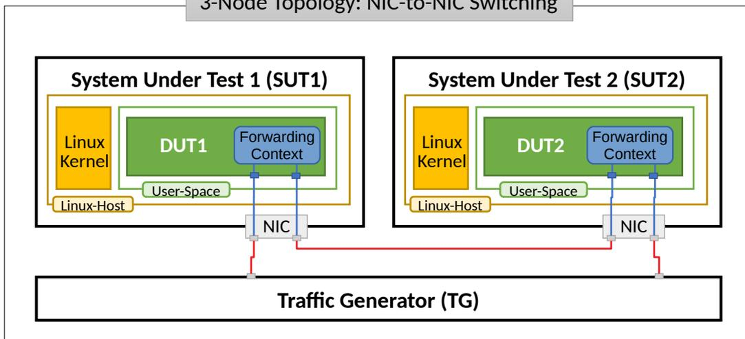
Server Systems Under Test (SUT) run VPP application in Linux user-mode as a Device Under Test (DUT). Server Traffic Generator (TG) runs T-Rex application. Physical connectivity between SUTs and TG is provided using different drivers and NIC models that need to be tested for performance (packet/bandwidth throughput and latency).
