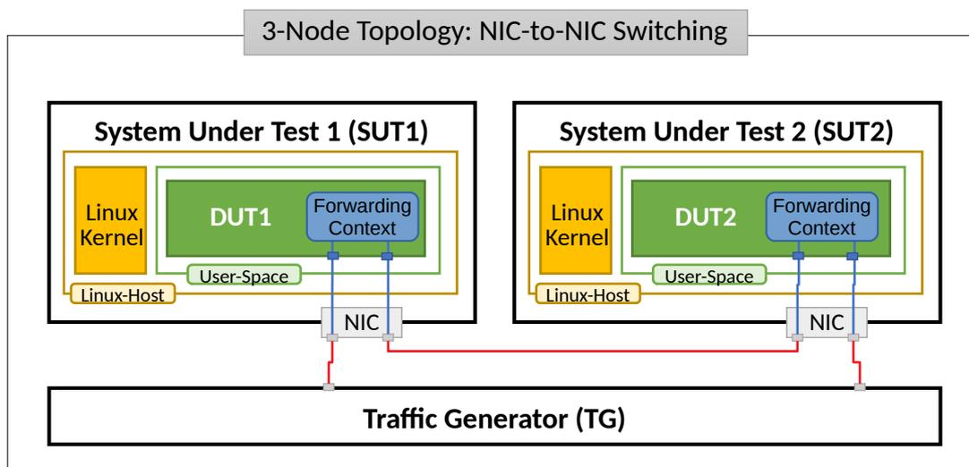
Server Systems Under Test (SUT) run DPDK Testpmd or L3fwd application in Linux user-mode as a Device Under Test (DUT). Server Traffic Generator (TG) runs T-Rex application. Physical connectivity between SUTs and TG is provided using different drivers and NIC models that need to be tested for performance (packet/bandwidth throughput and latency).
