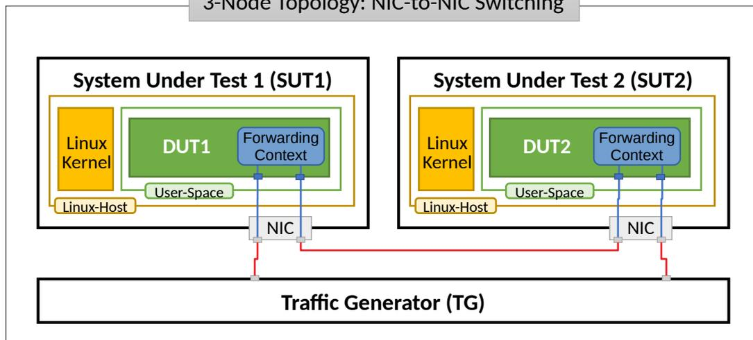
Server Systems Under Test (SUT) run DPDK Testpmd or L3fwd application in Linux user-mode as a Device Under Test (DUT). Server Traffic Generator (TG) runs T-Rex application. Physical connectivity between SUTs and TG is provided using different drivers and NIC models that need to be tested for performance (packet/bandwidth throughput and latency).
