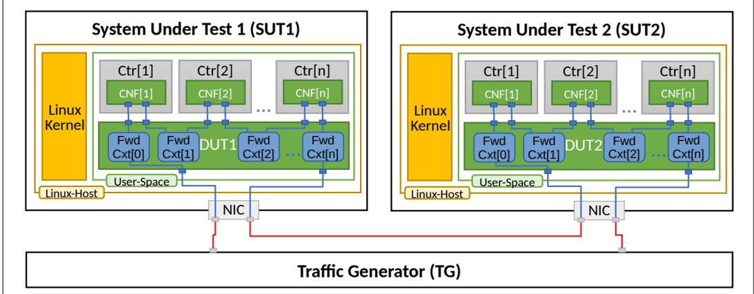
In “Chained” Container topologies, packets are switched by VPP DUT multiple times: twice for a single Container, three times for two Containers, N+1 times for N Containers. Hence the external throughput rates measured by TG and listed in this report must be multiplied by N+1 to represent the actual VPP DUT aggregate packet forwarding rate.
