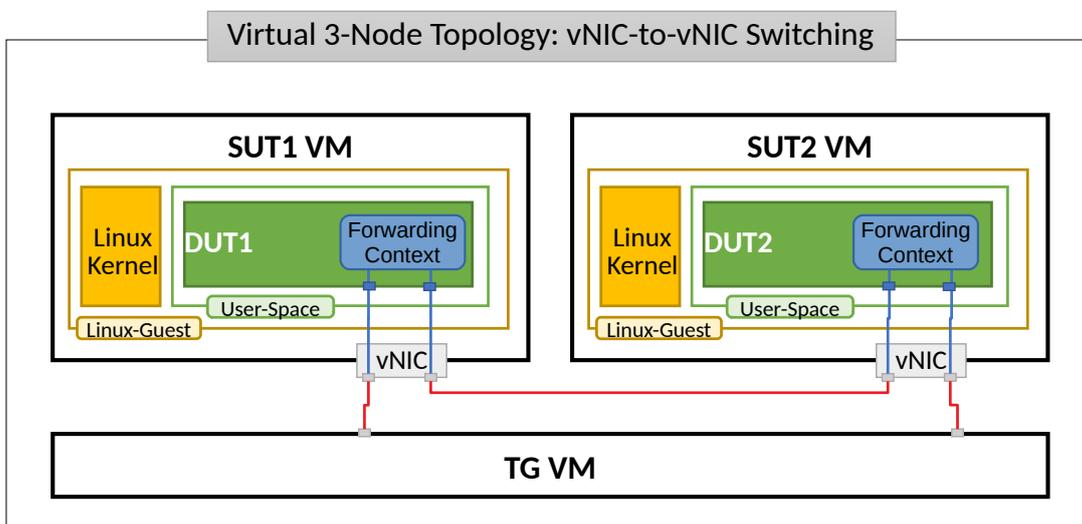
SUT1 and SUT2 are two VMs (running Ubuntu or Centos, depending on the test suite), TG is a Traffic Generator (running Ubuntu VM). SUTs run VPP SW application in Linux user-mode as a Device Under Test (DUT) within the VM. TG runs Scapy SW application as a packet Traffic Generator. Network connectivity between SUTs and to TG is provided using virtual NICs and VMs' virtio drivers.
