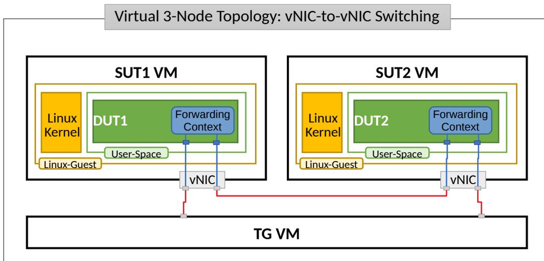
SUT1 and SUT2 are two VMs (running Ubuntu), TG is a Traffic Generator VM (running Ubuntu). SUTs run sample server-client application using the DMM libraries in Linux user- mode as a Device Under Test (DUT) within the VM. Currently TG node is not being used in DMM-CSIT. Network connectivity between SUTs and to TG is provided using virtual NICs and VMs' virtio drivers.
