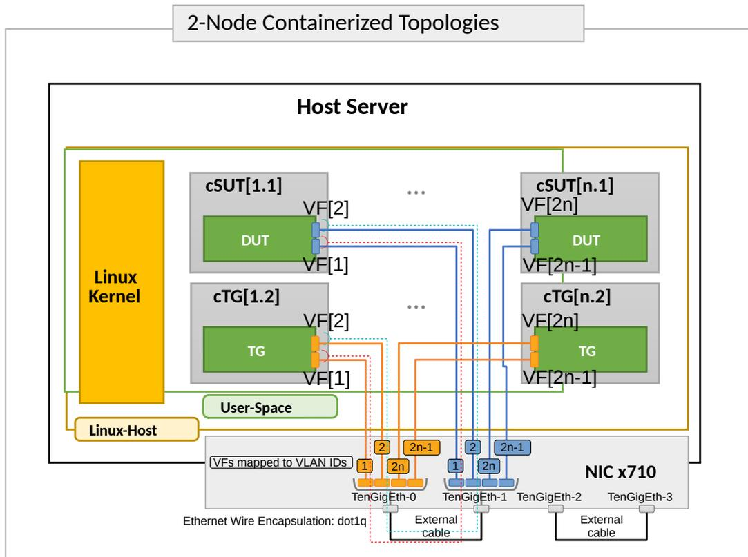
SUT1 is Docker Container (running Ubuntu, depending on the test suite), TG is a Traffic Generator (running Ubuntu Container). SUTs run VPP SW application in Linux user-mode as a Device Under Test (DUT) within the container. TG runs Scapy SW application as a packet Traffic Generator. Network connectivity between SUTs and to TG is provided using virtual function of physical NICs.
