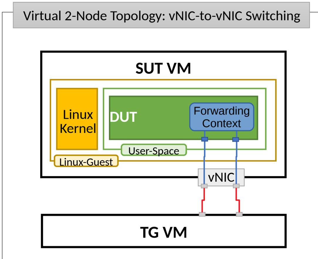
SUT (System Under Test) is a VM running Ubuntu Linux (or Centos, depending on the test suite), TG (Traffic Generator) is another VM running Ubuntu Linux. SUT VMs run HoneyComb management agent and VPP in Linux user-mode as a combined DUT (Device Under Test). TG runs Scapy application as a packet Traffic Generator. Virtual connectivity between SUT and TG is provided using virtual NICs using VMs' virtio drivers.
